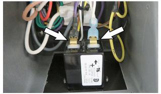
6. Connect the kit harness to the disconnected wire terminals. Plug diode into harness.
