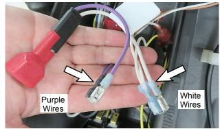
7. Reconnect wire terminals to the hour meter. Secure diode harness with cable-tie.
